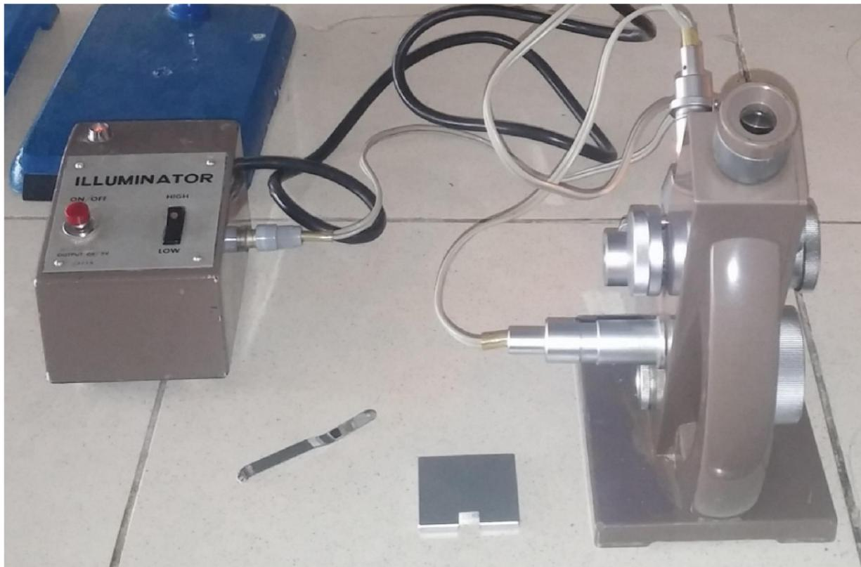
The lamps of the refractometer are first removed and after 1-2 drops of sample are dropped into the prism chamber, the lamps are put back and the refractive index is measured after looking through the eyepieces (Slide 8).
