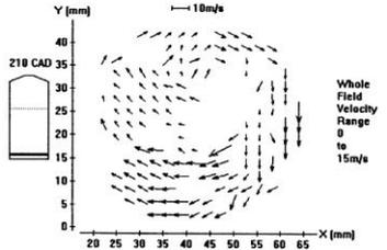
whole-body rotation or a significant out-of-plane velocity structure. Similar observations have been made in strong tumbling flows, where much of the flow momentum was contained in a swirl “tongue” that precessed around the cylinder volume [12,15]. The results here confirm that the detailed *temporal* and *spatial* structure of the flow must be considered when optimising fluid mechanical design for particular combustion strategies.
