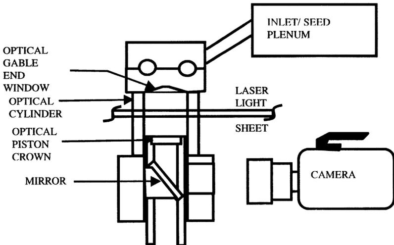
Fig. 2. The single cylinder optical engine showing optical access.
