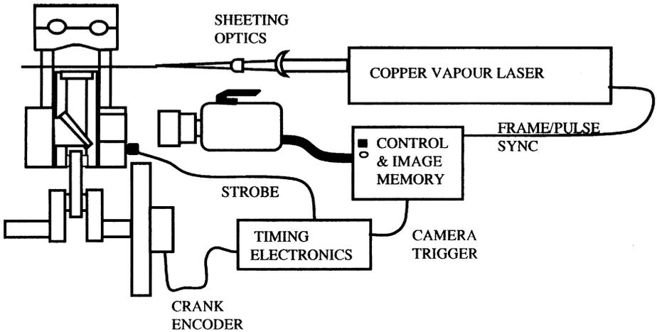
Fig. 1. Schematic of system layout.
