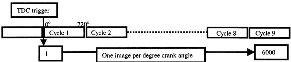
Fig. 3. Image recording scheme for cycle-resolved flow histories.
