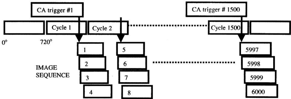
Fig. 4. Image recording scheme for study of cyclic variability at a particular crank angle.
