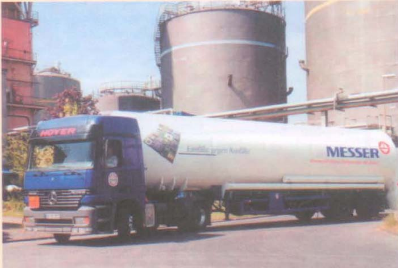
Tanker truck with a transport capacity of 40,000 liter of LH 2 Photo: Messer
