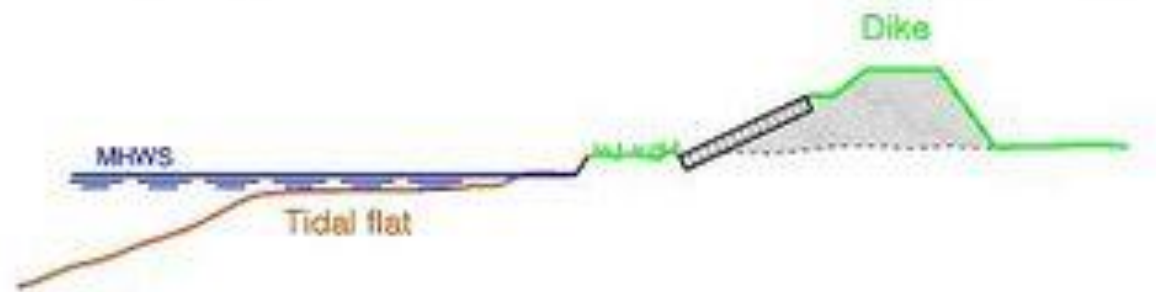
Gabion mattress revetment at foot of dike
