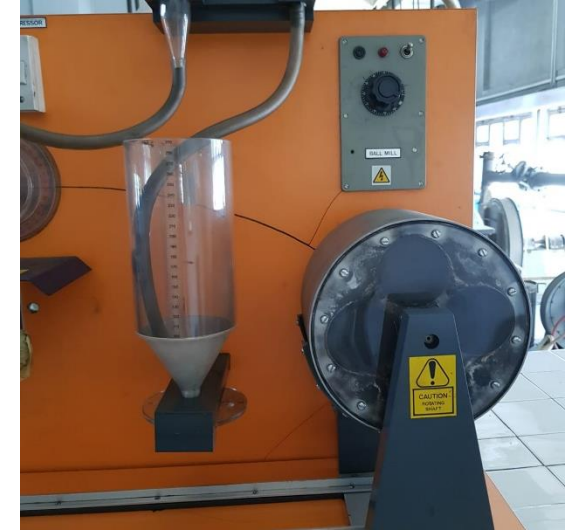
LHS : Tumbling Mixer | RHS : Ball Mill Grinder
