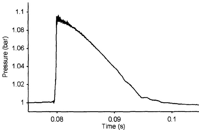
Figure 2. Discontinuity measured in a compression wave after travelling through a straight duct.
