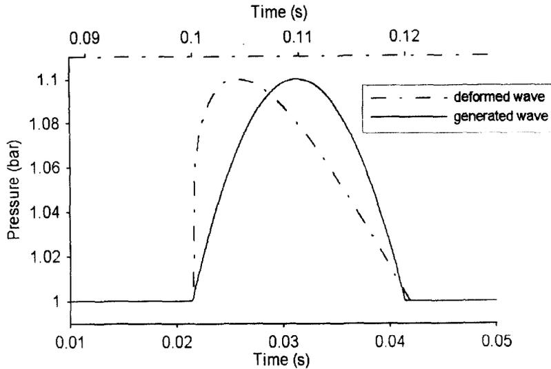
Figure 1. Numeric solution of a pressure evolution after travelling through a straight duct.
