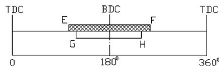
Fig. 2. Schematic of the port timing of the two stroke ICE with the methane mode combustion (1) Horizontal ordinate is the turning angle of the crankshaft; TDC: top dead center; BDC: bottom dead center; E: the open time of the air outlet valve; F: the close time of the air outlet valve; EF: the duration of the air outlet valve open; G: the open time of the scavenge port; H: the close time of the scavenge port; GH: the duration of the scavenge port open.
