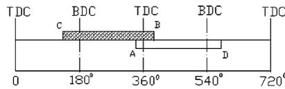
Fig. 1. Schematic of the port timing of the four stroke ICE with the methane mode combustion. Horizontal ordinate is the turning angle of the crankshaft; TDC: top dead center; BDC: bottom dead center; C: the open time of the air outlet valve; B: the close time of the air outlet valve; CB: the duration of the air outlet valve open; A: the open time of the air inlet valve; D: the close time of the air inlet valve; AD: the duration of the air inlet valve open.
