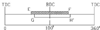
Fig. 3. Schematic of the port timing of the two stroke ICE with the methane mode combustion (2) Horizontal ordinate is the turning angle of the crankshaft; TDC: top dead center; BDC: bottom dead center; E: the open time of the air outlet valve; F: the close time of the air outlet valve; EF: the duration time of the air outlet valve open; G: the open time of the scavenge port; H': the close time of the scavenge port; GH': the duration of the scavenge port open.
