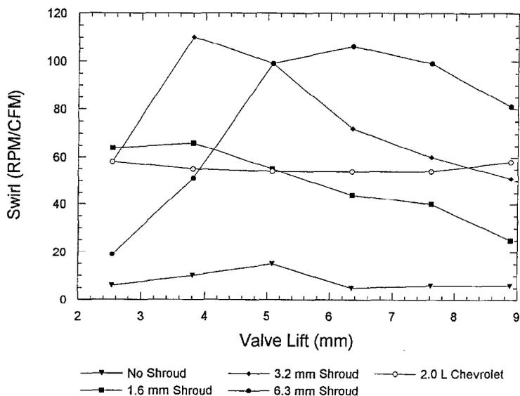
Fig. 1. Effect of valve lift on swirl.
