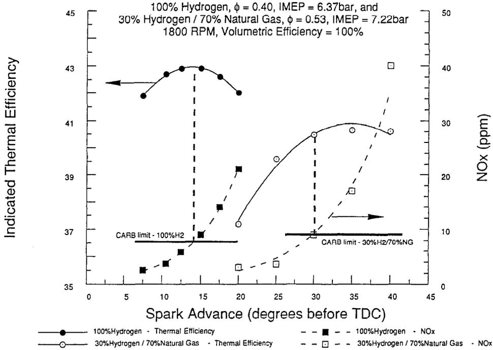
Fig. 6. Indicated thermal efficiency and NO<sub>x</sub> vs spark advance. 100% Hydrogen,  $\phi = 0.4$ , IMEP = 6.37 bar, and 30% hydrogen/70% natural gas,  $\phi = 0.53$ , IMEP = 7.22 bar, 1800 rpm, volumetric efficiency = 100%.
