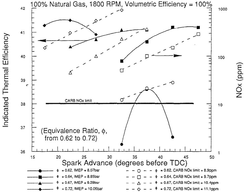
Fig. 4. Indicated thermal efficiency and NO<sub>x</sub> vs spark advance. 100% Natural gas, 1800 rpm, volumetric efficiency = 100%.
