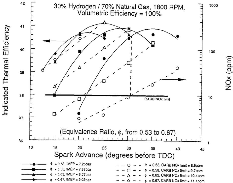
Fig. 5. Indicated thermal efficiency and NO<sub>x</sub> vs spark advance. 30% Hydrogen/70% natural gas, 1800 rpm, volumetric efficiency = 100%.
