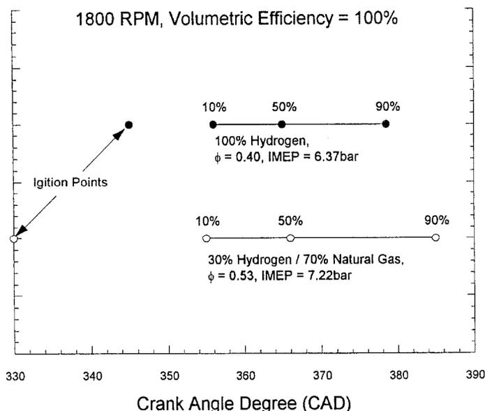
Fig. 8. Burn duration at specific crank angle degrees.
