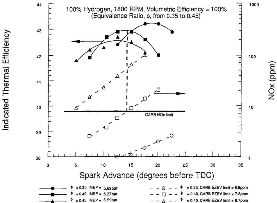
Fig. 3. Indicated thermal efficiency and NO<sub>x</sub> vs spark advance. 100% Hydrogen, 1800 rpm, volumetric efficiency = 100%.
