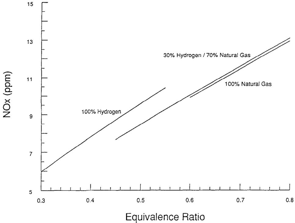
Fig. 2. NO<sub>x</sub> limit vs equivalence ratio to meet proposed CARB EZEV Standard for vehicle attaining 60 mpg.
