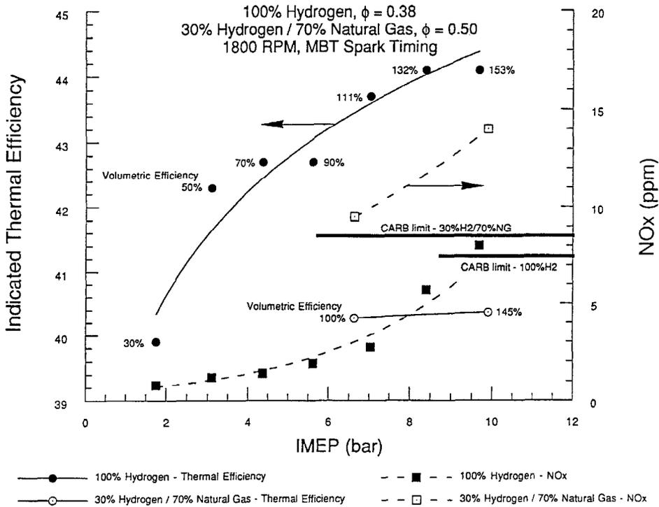
Fig. 7. Indicated thermal efficiency and NO<sub>x</sub> vs indicated mean effective pressure. 100% Hydrogen,  $\phi = 0.38$ , 30% hydrogen/70% natural gas,  $\phi = 0.50$ , 1800 rpm, MBT spark timing.
