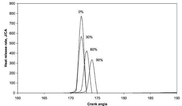
Fig. 18. Calculated heat release rate with varying quantity of N<sub>2</sub>.
