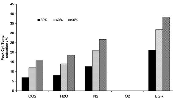
Fig. 15. Effect of added gases on peak cylinder temperature reduction.
