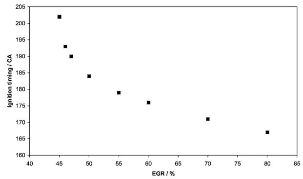
Fig. 4. Calculated effect of EGR at 800 K on the ignition timing of HCCI combustion.
