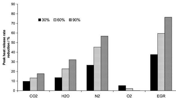
Fig. 21. Effect of added gases on heat release rate reduction.
