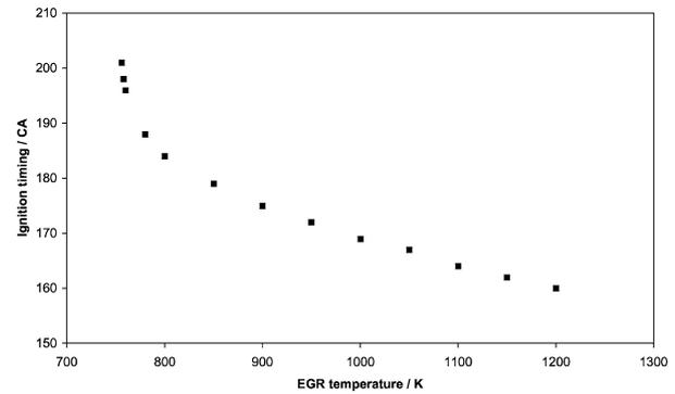
Fig. 8. Calculated effect of EGR temperature on ignition timing.
