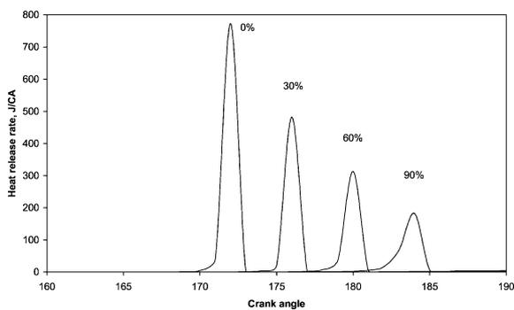
Fig. 20. Calculated heat release rate with varying quantity of EGR.
