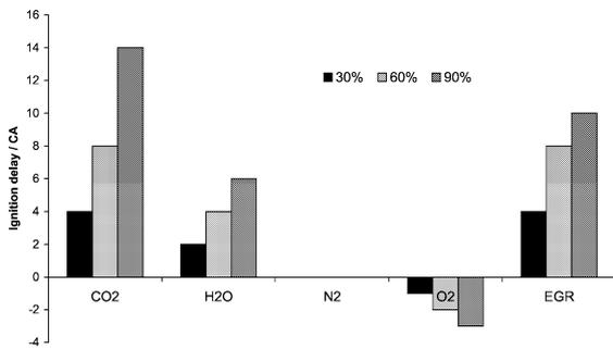
Fig. 14. Effect of added gases on ignition delay of HCCI combustion.
