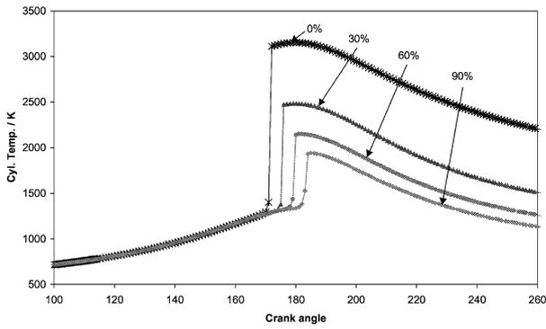
Fig. 13. Calculated cylinder temperature with varying quantity of simulated EGR.
