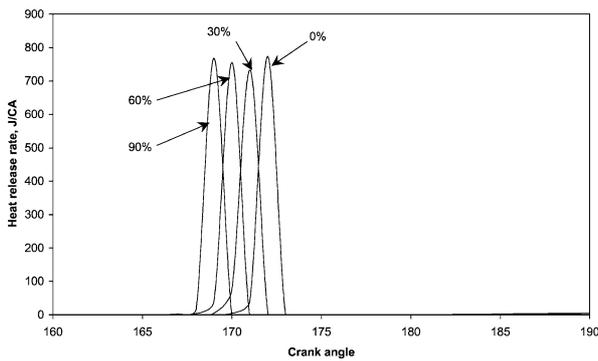
Fig. 19. Calculated heat release rate with varying quantity of O<sub>2</sub>.
