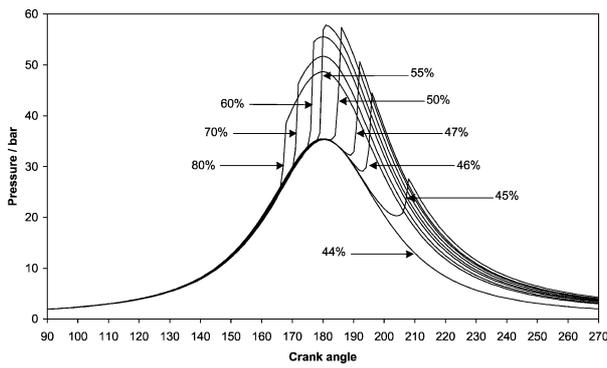
Fig. 2. Calculated cylinder pressure with varying quantity of EGR at 800 K.
