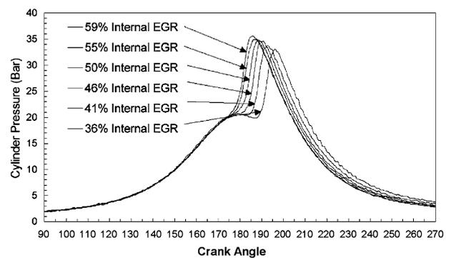
Fig. 1. Cylinder pressure trace data for HCCI with different quantities of internal EGR [8].
