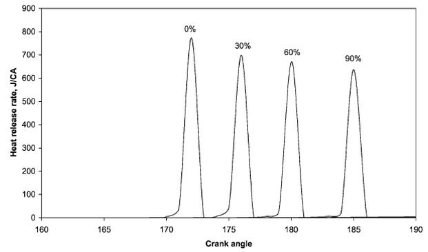
Fig. 16. Calculated heat release rate with varying quantity of CO<sub>2</sub>.
