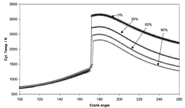
Fig. 11. Calculated cylinder temperature with varying quantity of N<sub>2</sub>.
