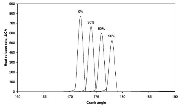
Fig. 17. Calculated heat release rate with varying quantity of H<sub>2</sub>O.
