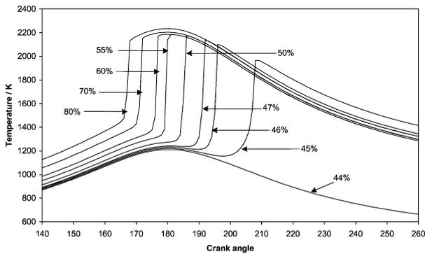
Fig. 3. Calculated cylinder temperature with varying quantity of EGR at 800 K.
