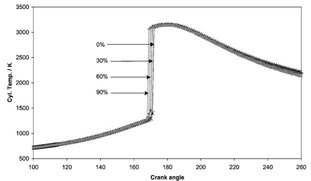
Fig. 12. Calculated cylinder temperature with varying quantity of O<sub>2</sub>.
