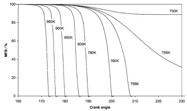
Fig. 7. Mass fraction burned with 50% of EGR at varying temperature.
