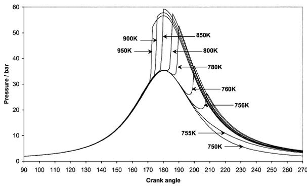
Fig. 5. Calculated cylinder pressure with 50% of EGR at varying temperature.
