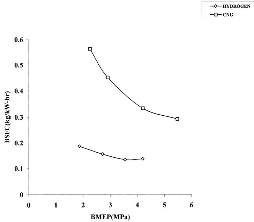
Fig. 12. Variation of brake-specific fuel consumption with brake mean effective pressure at 2400 rpm.
