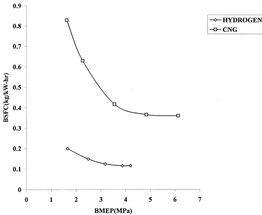
Fig. 11. Variation of brake-specific fuel consumption with brake mean effective pressure at 2200 rpm.
