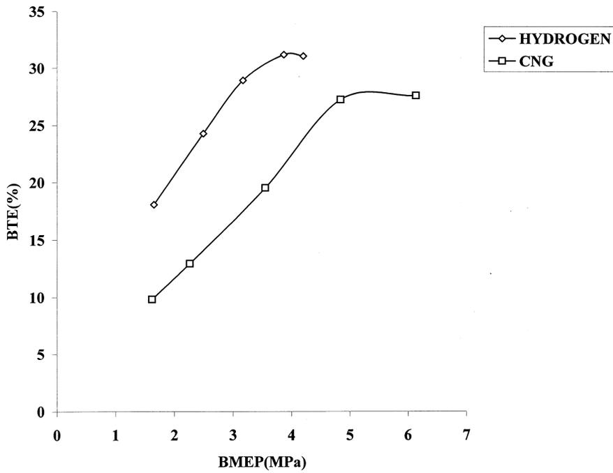
Fig. 7. Variation of brake thermal efficiency with brake mean-effective pressure at 2200 rpm.
