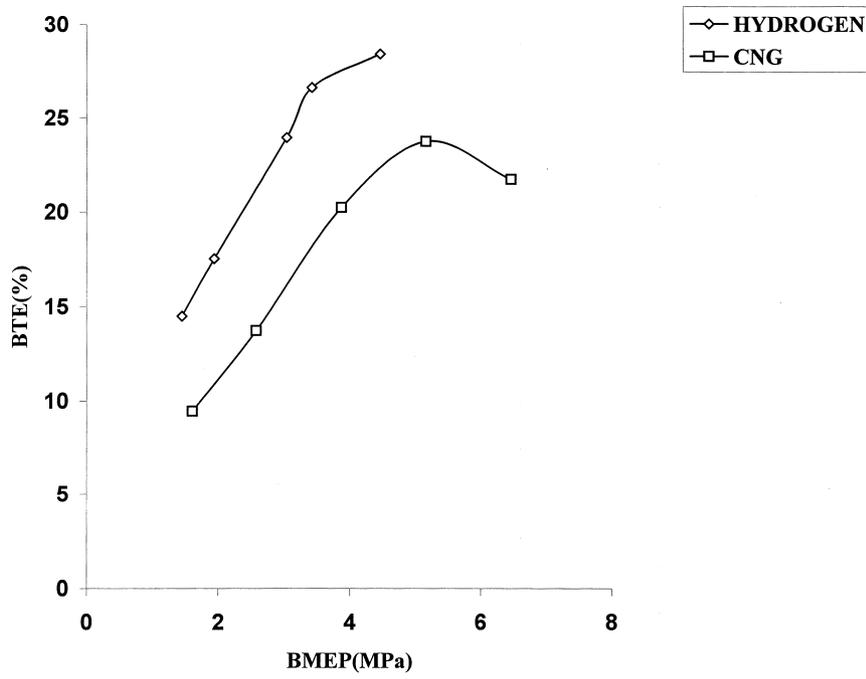
Fig. 6. Variation of brake thermal efficiency with brake mean-effective pressure at 2000 rpm.
