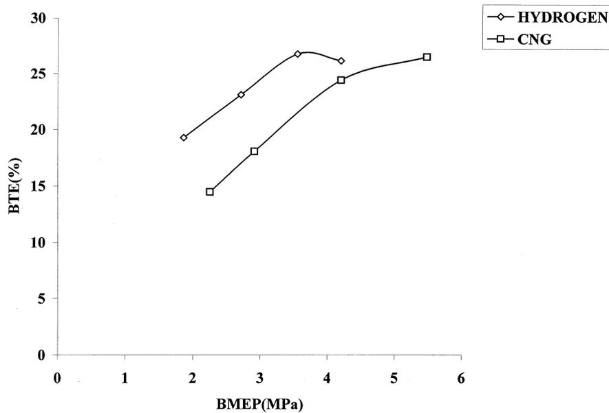
Fig. 8. Variation of brake thermal efficiency with brake mean-effective pressure at 2400 rpm.
