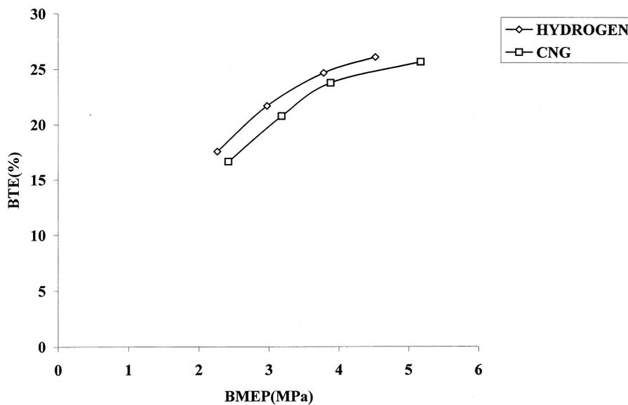
Fig. 9. Variation of brake thermal efficiency with brake mean-effective pressure at 2600 rpm.
