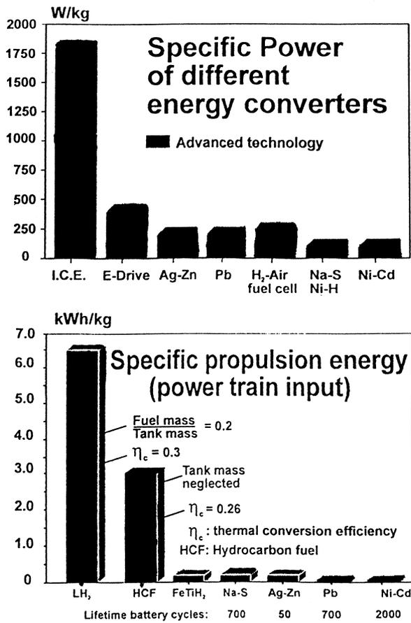
Fig. 1. Power-to-mass and energy-to-mass ratio of vehicular propulsion. Fuel mass, drive engine, fuel storage and energy converter included.
