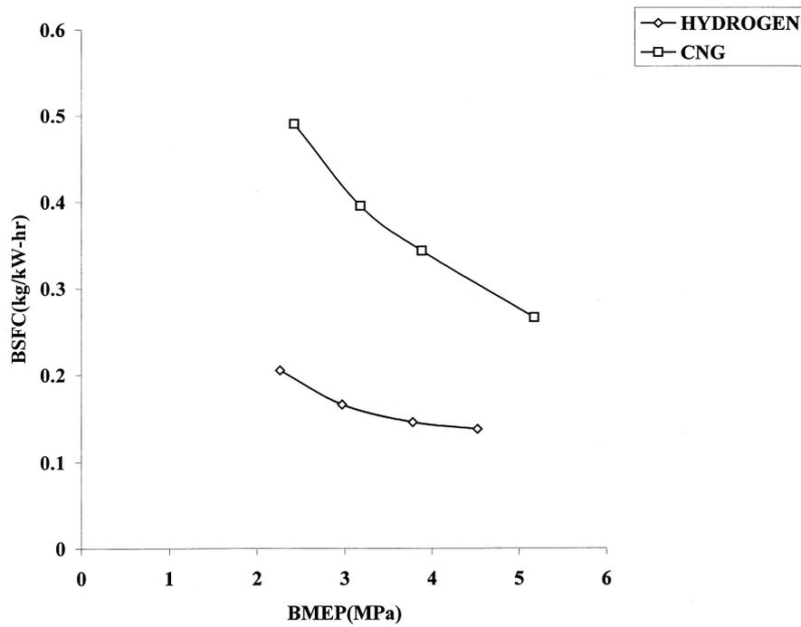
Fig. 13. Variation of brake-specific fuel consumption with brake mean effective pressure at 2600 rpm.
