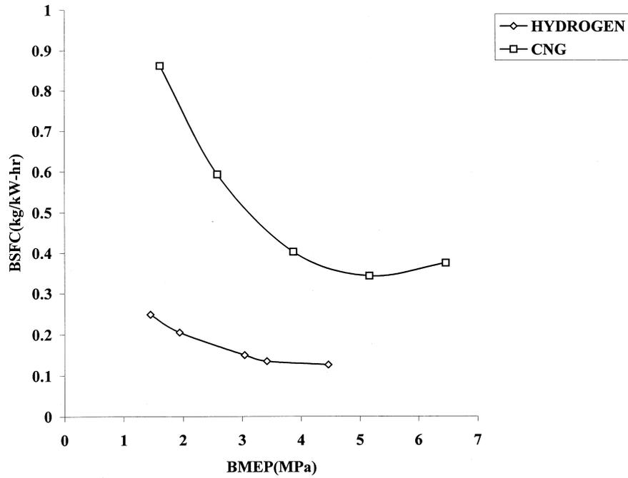
Fig. 10. Variation of brake-specific fuel consumption with brake mean effective pressure at 2000 rpm.
