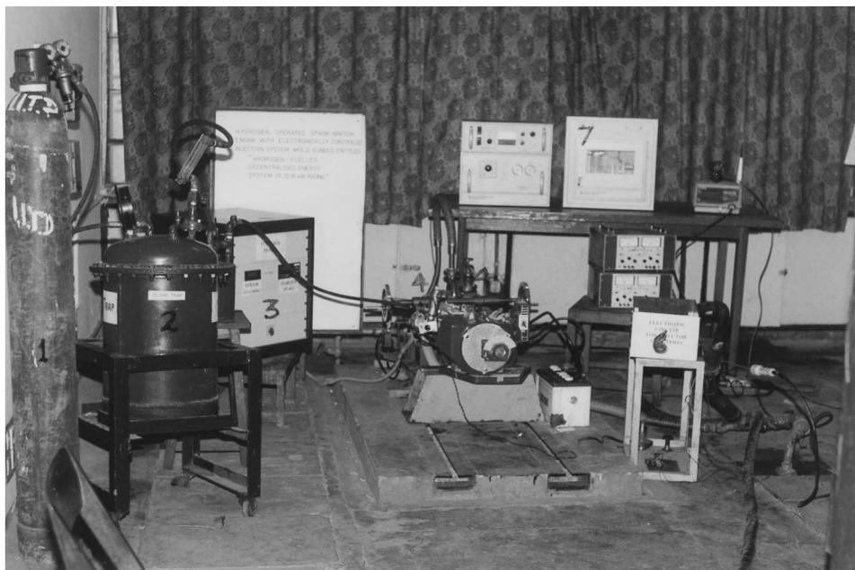
Fig. 5. Hydrogen operated SI engine with electronically controlled injection system. 1. Hydrogen cylinder; 2. flame trap; 3. control panel; 4. SI engine coupled with hydraulic dynamometer; 5. injector; 6. electronic mechanism for injector actuation; 7. chemiluminescent  $\text{NO}_x$  analyzer; 8. non-dispersive infrared CO-HC gas analyzer.
