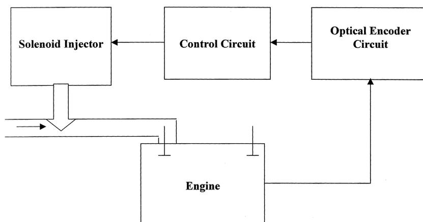
Fig. 3. Electronically controlled injection system.
